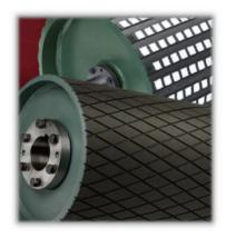
**Pulley Lagging:** protecting the pulley shell from wear damage, and extending the pulley's service life. The lagging also increases the friction between the conveyor belt and the pulley to reduce belt slippage, and minimizes the buildup of bulk material, water, ice, or snow.
