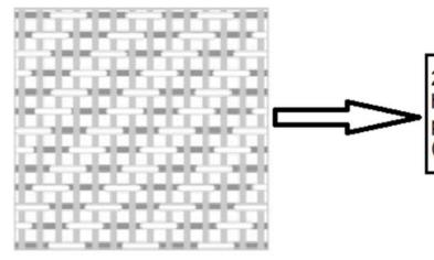
2x2 broken twill fabric weave which has each warp (longitudinal) thread passing over/under two weft (transverse) threads at a time.
